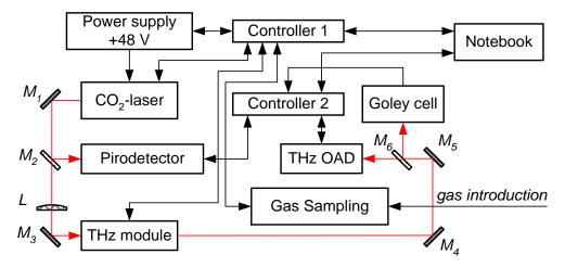
Figure 8. THz Laser block diagram. M1, M3, M4, M5 – deflecting mirrors, M2, M6 – beam splitters, L - focusing lens.
