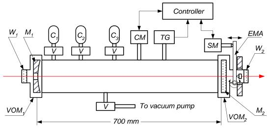
Figure 9. THz module.  $W_1$  – ZnSe window,  $W_2$  – TPX window, V – vacuum valve,  $C_1 - C_3$  – chambers with a gain medium,  $VOM_1$ ,  $VOM_2$  – vacuum optical mounts,  $M_1$ ,  $M_2$  – laser cavity mirrors, CM – capacitance manometer, TG – thermocouple gauge, SM – stepper motor, EMA – electro-mechanical actuator.
